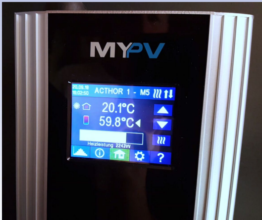
Figure 4: AC•THOR display with status indicators
