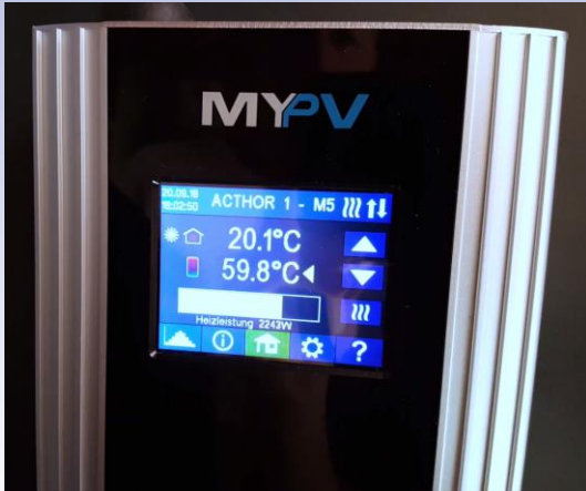
Figure 4: AC•THOR display with status indicators
