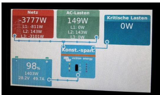
The AC•THOR receives the information of the surplus from the Victron Color Control GX by Modbus TCP via network. Control is possible with both single-phase and three-phase house connections.
