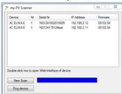
5. Are there more AC ELWA-Es in the network, the desired device can be determined by the serial number (lateral on the case)!
